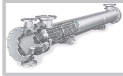
Straight-tube, removable bundle exchangers made from standard components. Floating tube sheet for seal leak detection and easy maintenance. Diameters from 3" (7.62 cm) to 42" (106.68 cm). ASME, API, TEMA, ABS and other codes available.
