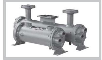
General purpose exchangers designed to cool oil, compressed air and other industrial fluids. A variety of constructions, port configurations and materials are available. ASME and TEMA-C available. Diameters from 3" (7.62 cm) to 12" (30.48 cm).
